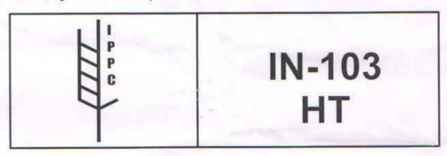
Foot Note: Markings should be according to the model shown above (12 x 6 cm), legible, permanent, not transferable, placed in a visible location and preferably marked by a stencil with black ink. The letter size should be a minimum of 2.5 cm. Recycled, remanufactured or repaired wood packaging material should be re-certified and re-marked. All components of such material should have been treated.
